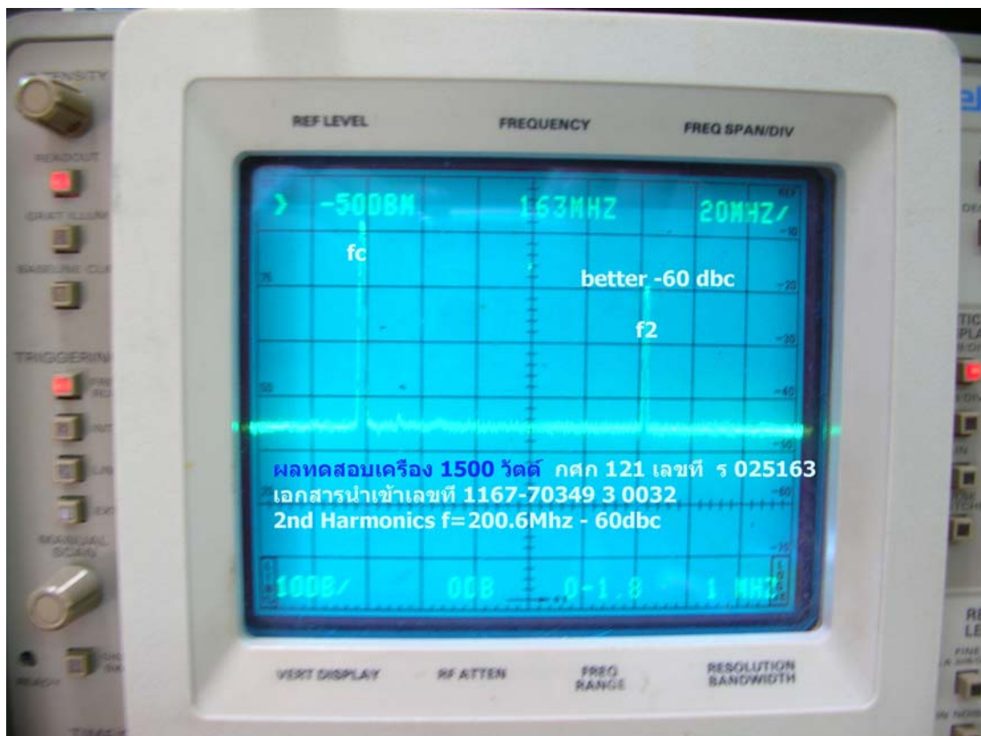
2 nd Harmonics Test @ 1500Watt better -60dBc
